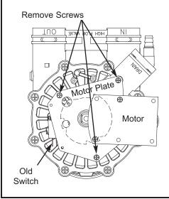
2. Remove screws holding old switch. Save screws and discard old switch. Install new switch using the same screws. If the old switch did not have a lever, the new switch will be installed in a different spot (see below).
