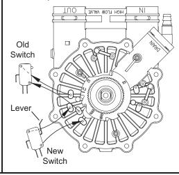
**3.** Make sure new switch is installed where shown below, with lever toward the cam. Plug cable into switch and reinstall the motor plate (removed in Step 1).
