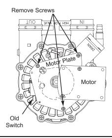
2. Remove screws holding old switch. Save screws and discard old switch. Install new switch using the same screws. If the old switch did not have a lever, the new switch will be installed in a different spot (see below).
