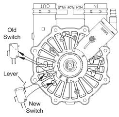
**3.** Make sure new switch is installed where shown below, with lever toward the cam. Plug cable into switch and reinstall the motor plate (removed in Step 1).
