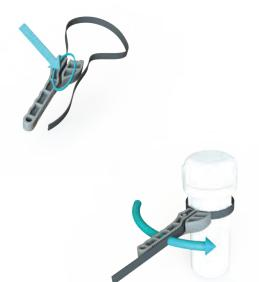
5. Turn wrench to the right/counterclockwise to tighten
