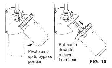
2. Pull the sump downward out of the head.
