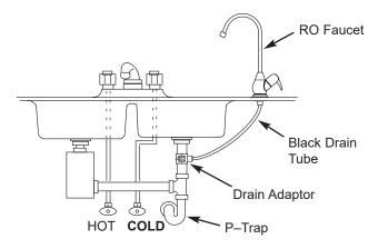
IMPORTANT: Do not install drain adaptor below the P-Trap.
