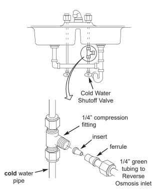
Cold Water Supply Connection (using compression fitting - not included)
